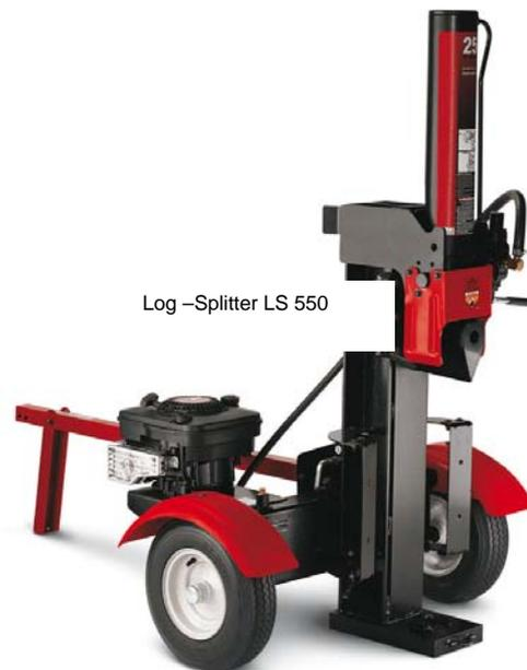
The MTD log-splitter LS 550 works with a pressure of up to 25 tons. Work is possible in a horizontal, as well as a vertical position. A cast-iron splitting wedge and the powerful Briggs & Stratton motor allow you to split pieces of wood with a length of up to 63,5 cm.
