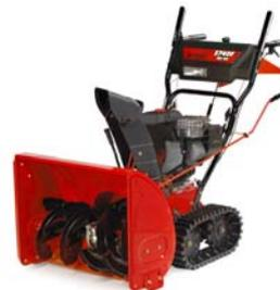
All of the two-stage machines have skids. With them you can adjust the working height in order to clear snow on gravel, lawn and rough terrain without damaging the ground or the machine. Most of the two-stage models can be equipped optionally with a dozer blade.
